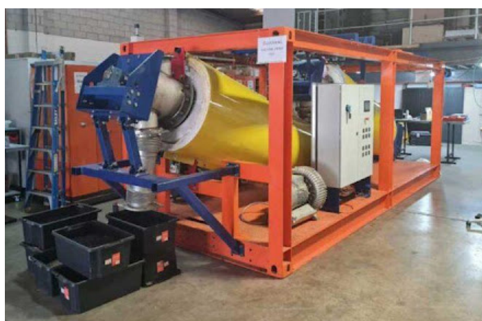
A Patriot pyrolysis reactor that turns woodchip into syngas and biochar.
